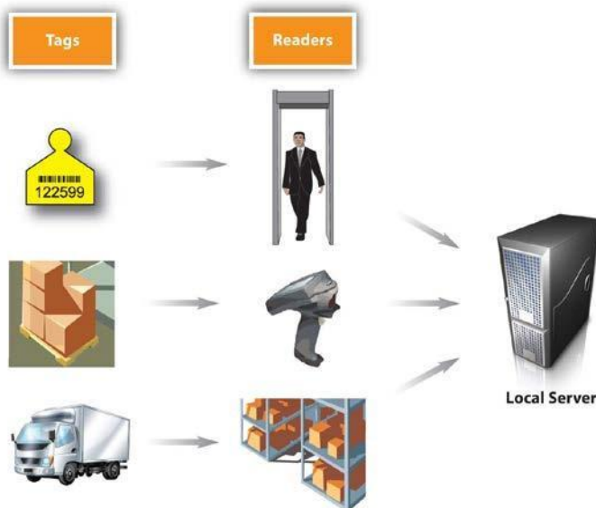
Figure 9.8 How RFID Tagging Works
